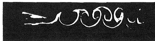
Fig. 7(b) Flow visualization of Bratt for a NACA 0015 airfoil
